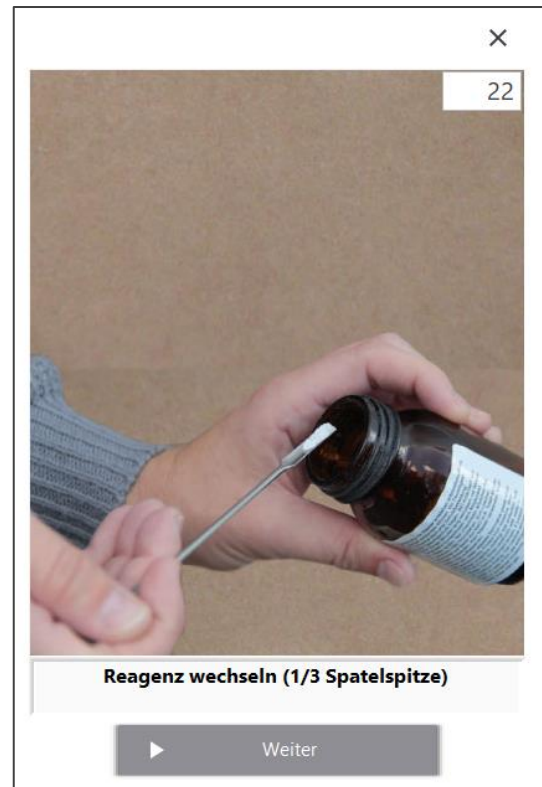
Using the spoon-shaped end of the spatula, take the reagent (about 1/3 of the spoon area) and fill the reagent bed.
