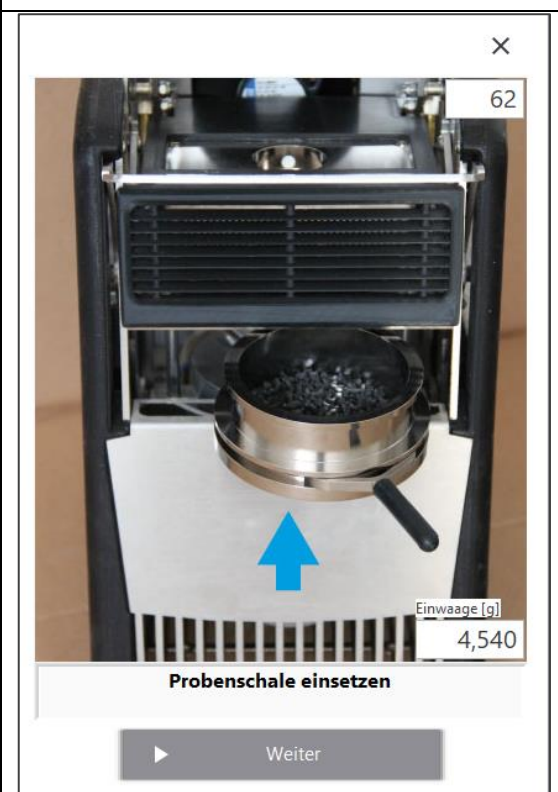
Insert the sample tray. Make sure the bottom edge of the tray is over the heater plate
