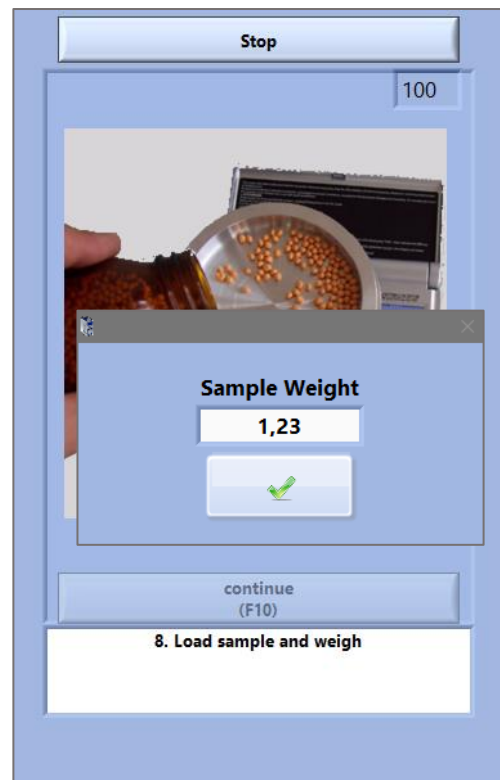
Fill in the sample material. Enter the weight in grams. Click on "Continue".
