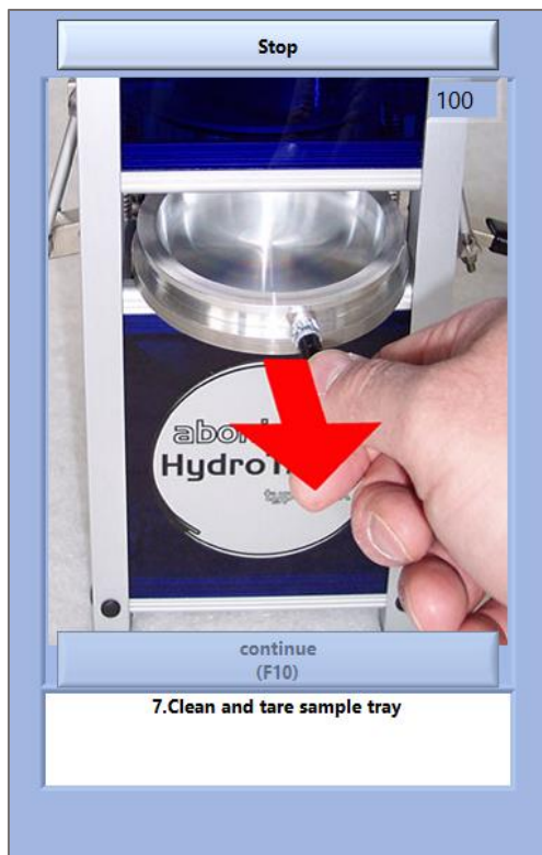
Remove the sample tray and dispose the sample material of the former test. Place the sample tray on the balance and tare it.
