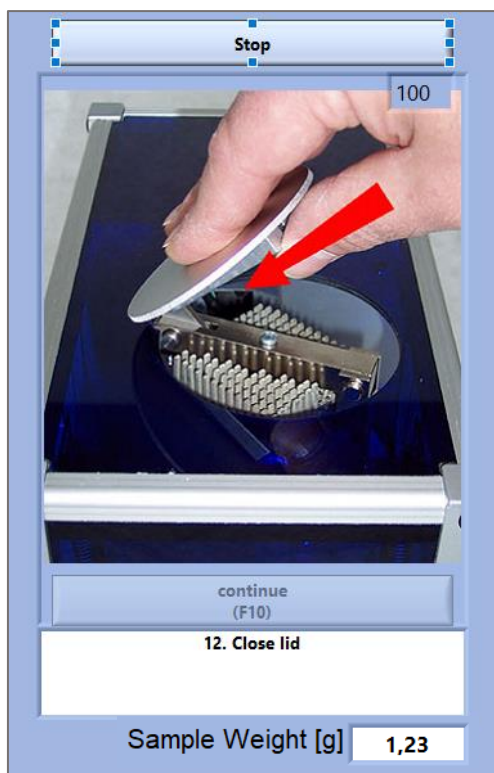
Close reactor lid. Take care the clasp is properly locked.
